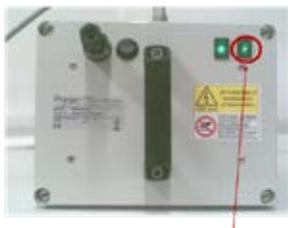
1. Turn off the device using the lighted green O/I switch, moving it to the 0 position
