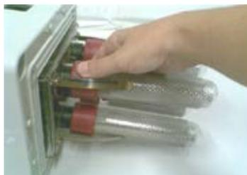
6. Remove the mesh (R) from the outside of the tube. If the operation is difficult, lightly rotate the mesh around the quartz condenser.
